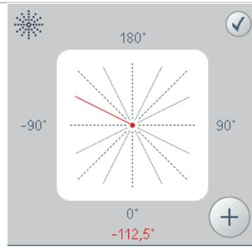
**10** Touch the "plus" 6 times to add six stitches in the direction of  $-112.5^\circ$
