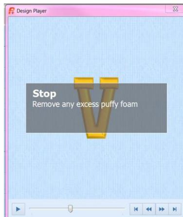
Using color 2, the foam is stitched down and a satin stitch is embroidered on top of the foam. The machine stops to remove excess foam.
